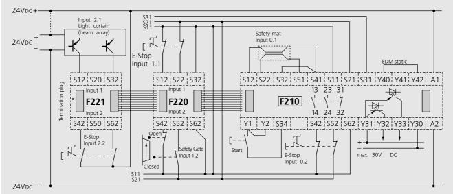
F221 application: Input 1 activated via Light-curtain, Input 2 : dual-channel E-Stop via supply voltage without crossfault monitoring
