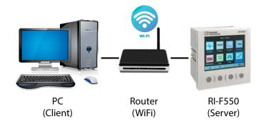
The parameters of the RI-A5WiFi module can also be configured through special software. The RI-F500 Series analysers are equipped with a RS485 interface and can be connected to a PC through a RS232(USB) / RS485 conversion device. See the user manual for more information.
