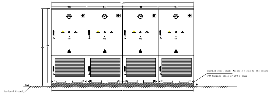
Front view of hardened Ground (channel steel foundation)
