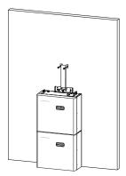
Step 3: Fit the inverter on to the bracket. Take care to ensure the rear tang correctly engages with the bracket.
