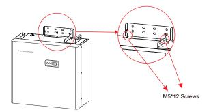
Step 2: Place the battery module against the wall and mark the 4 holes indicated below that are to be drilled. Using an 8mm Ø masonry drill bit, drill 4 x holes approximately 70mm depth. Gently tap supplied nylon wall plugs in to the holes.
