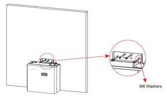
Step 4: Repeat steps 1-3 for any additional batteries. Please note, for installs with more than 2 battery modules it will be necessary to start a second battery stack to the right-hand side of the first. **See full user manual for mandatory separation distances.**
