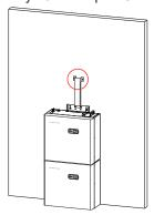
Step 2: Remove any debris. Secure the inverter bracket to the wall using the supplied screws (2 from battery installation + washers for the bottom holes and 2 without washers for the top holes).
