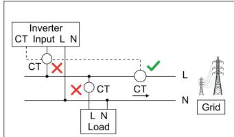
In order for the system to work correctly, a load sensing current transformer MUST be installed. Alternatively, an external Modbus meter may be used. Meter installation is outside of the scope of this guide. Please refer to the full user manual if meter measurement is needed.
