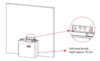
Step 3: Remove any debris. Secure the battery module to the wall using the supplied mounting screws and M6 washers. On the last battery module of the stack, leave the two central screws unfitted and proceed to the next section for **Inverter Installation**
