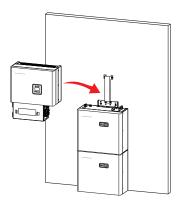
Step 4: Loosely fit the 4xM5x12mm screws through the battery brackets in to the inverter. Before tightening the screws position the inverter so that the removable inverter cover fits flush with the battery front panel(s). Do not fit the cover at this stage.
