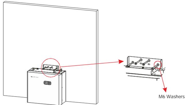
Step 4: Repeat steps 1-3 for any additional batteries. Please note, for installs with more than 2 battery modules it will be necessary to start a second battery stack to the right-hand side of the first.
