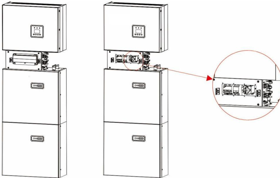
Figure 17 The external PV switch.
