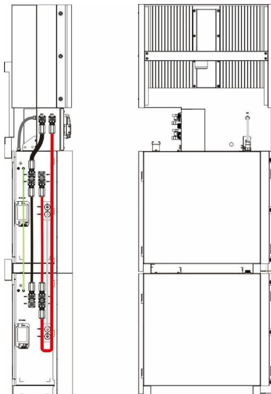
8. Close the battery covers and connect the PV -MC4 connectors to the system (connection on both sides). Also, connect all AC cables, the meter communications cable METER, and the Ethernet cable LAN. Then close the cable box cover. The installation is now complete.
