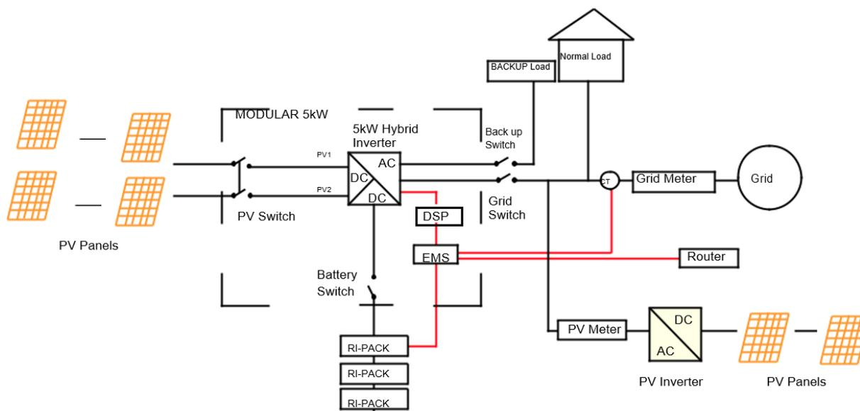
Figure 16 Hybrid-coupled system
