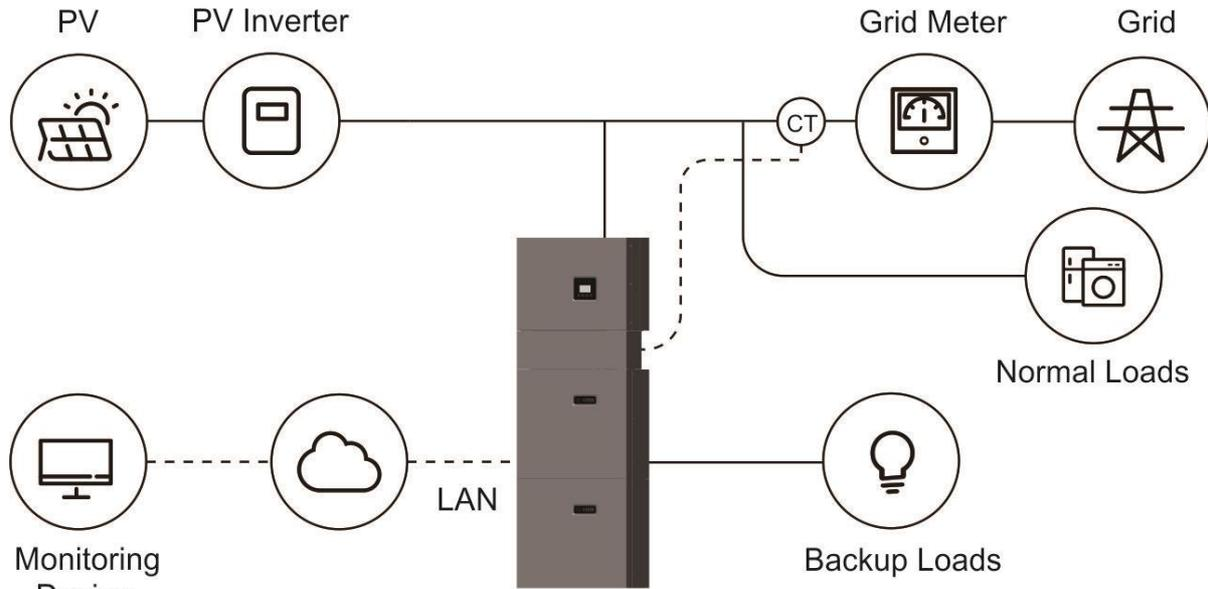
Figure 2 AC-coupled Storage System–Scheme
