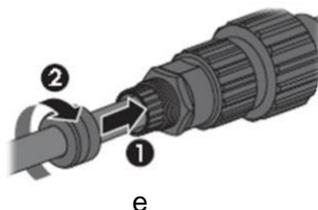
f. Assembly the plug shell adapter as below picture, push the adapter and shell by hand until a “Click” is heard or felt.
