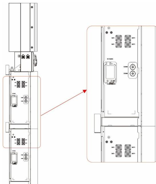
7. Connect the power cables of the bottom battery from Step 4 to the side terminals of the top battery. Make sure that red connects to red and black connects to black.
