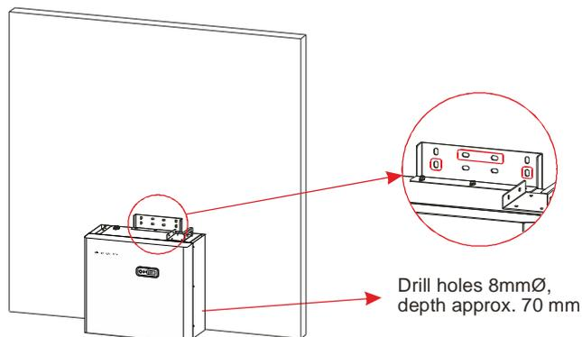
Step 3: Remove any debris. Secure the battery module to the wall using the supplied mounting screws and M6 washers. On the last battery module of the stack, leave the two central screws unfitted and proceed to the next section for **Inverter Installation**
