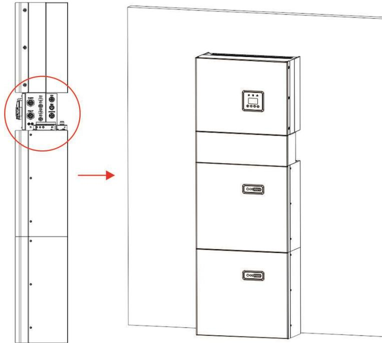
If you connect more than 2 battery modules to the system, only install the additional batteries 5-6 (third module) on the side of the system. You can connect up to 6 batteries (three modules), each 2 batteries are mounted on top of each other.
