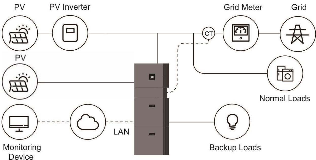
Figure 3 AC and DC (Hybrid)-coupled Storage System–Scheme
