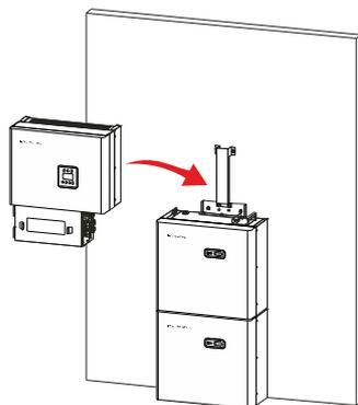
Step 4: Loosely fit the 4xM5x12mm screws through the battery brackets in to the inverter. Before tightening the screws position the inverter so that the removable inverter cover fits flush with the battery front panel(s). Do not fit the cover at this stage.
