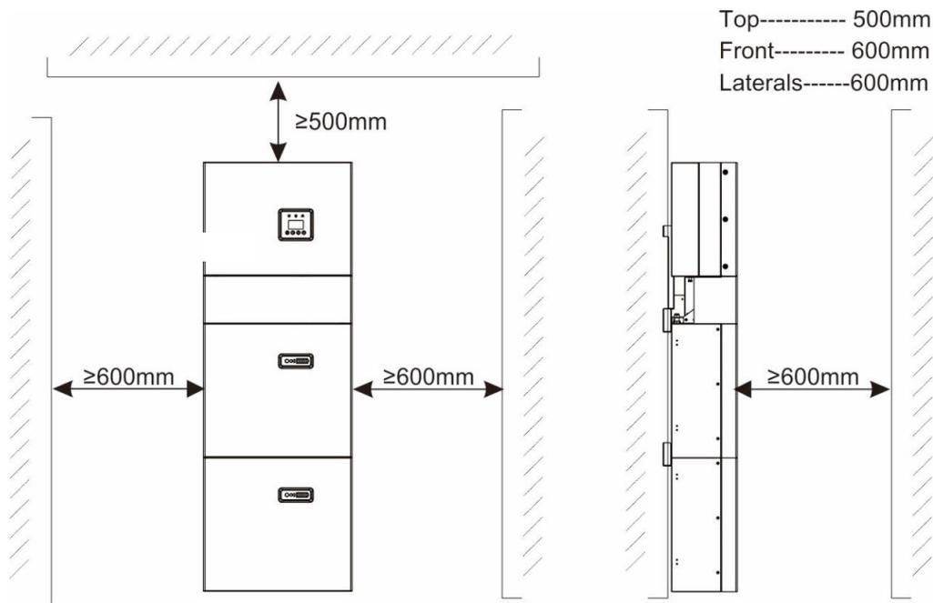
Figure 11 Limited Distance of Installation to Neighboring Objects
