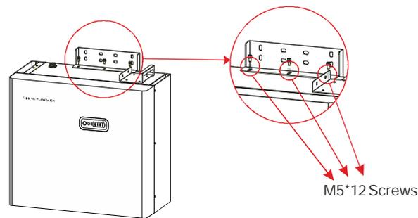
Step 2: Place the battery module against the wall and mark the 4 holes indicated below that are to be drilled. Using an 8mm Ø masonry drill bit, drill 4 x holes approximately 70mm depth. Gently tap supplied nylon wall plugs in to the holes.
