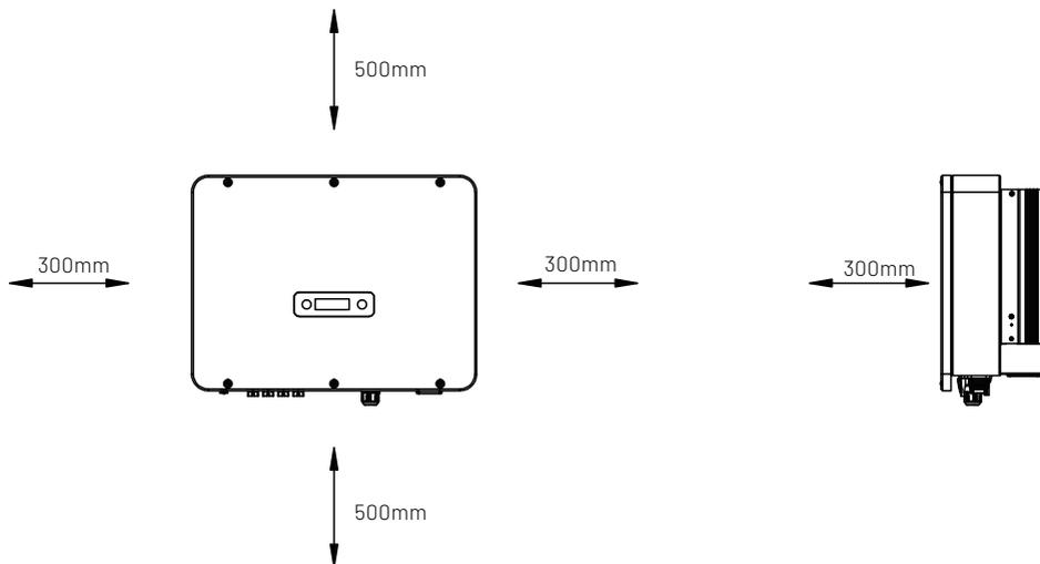
Figure 3-3 Distance required of Invertors
