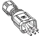
5) The cables are inserted into the terminal according to the wire sequence (L1/L2/L3/N/PE), so that the insulating terminal is flush with the surface of the terminal, and the crimping screw torque is  $2.0 \pm 0.1 \text{N}\cdot\text{m}$ .
