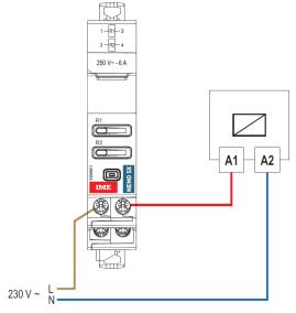
**Note:** whatever the configuration given to the Nemo SX Multifunction command module, local command of the module is still possible pushing on the 2 button on the front face of the module;
