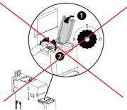
. It is not necessary to address the Nemo SX modules. The track wheel must be left in default position "0".
