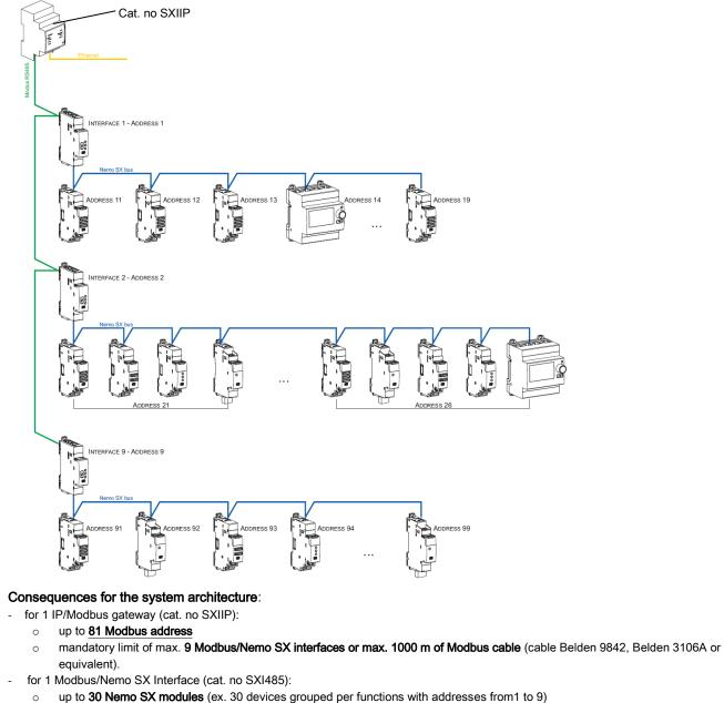
**Note:** with local addressing, the Modbus/Nemo SX interface, does the automatic detection of modules (characteristics, functions, configuration...)
