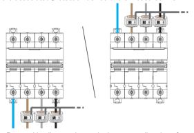
. Rogowski coils must be put in the correct direction of current flow (arrow drawing on the  ${
