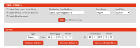
The "Report" section, contains the main controls of the reporting function. As a first step, set the time period, typically "from"... "to", of which retrieving the consumption data.
