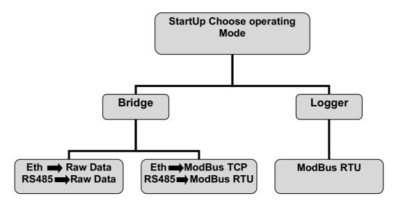
**Bridge with Raw Data**: any protocol can be transported over ETHERNET without any further manipulation. Modbus over TCP is the way to carry the Modbus RTU protocol as if it were transmitted on a normal RS485 line
