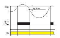
Monitoring relay PRI-32 serves to monitor current level in single phase AC circuits. Due to its fluent adjustment of release current, it is predestined for applications with necessity of current flow indication, and can be used as precedence relay. Output relay is off in normal state. In case the set current level is exceeded, it switches. Multivoltage supply is an advantage.
