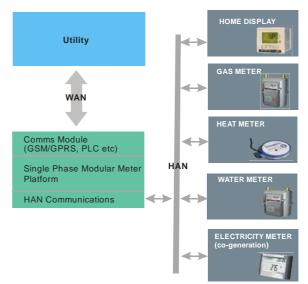
The HAN allows any remote meter to be read directly by the Utility or to be viewed on the Home Display.
