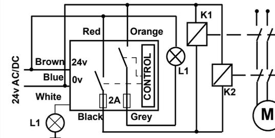
\* To protect safety outputs (internal 2A fuse) , you can use external 1.6A fast fuse.
